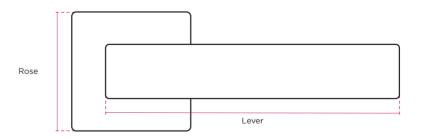
Levers are unsprung & require heavy duty latch or lock.
