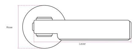
Levers are unsprung & require heavy duty latch or lock.
