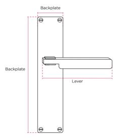
Levers are unsprung & require heavy duty latch or lock. Available as Latch, Lock, Euro Profile or Bathroom Function
