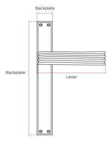
Levers are unsprung & require heavy duty latch or lock. Available as Latch, Lock, Euro Profile or Bathroom Function
