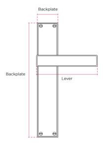
Levers are unsprung & require heavy duty latch or lock. Available as Latch, Lock, Euro Profile or Bathroom Function
