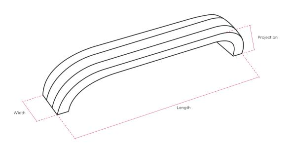
Fixings: Supplied 2x M4 x 30mm machine bolts
