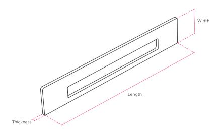
Width Thickness Length 48mm 300mm 6mm
